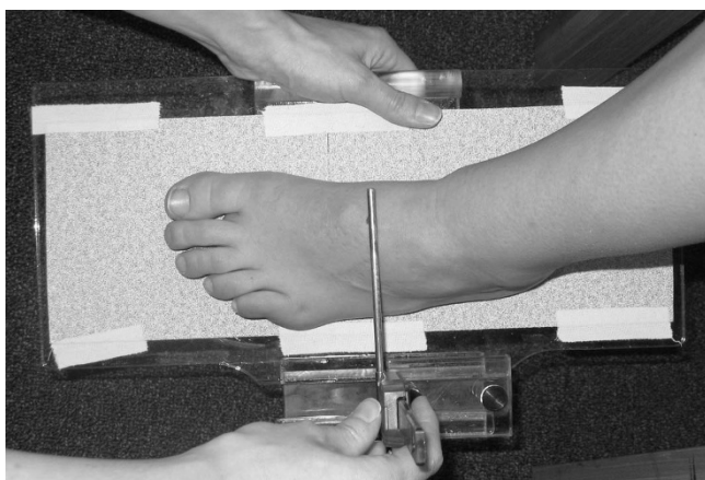
Figure 2 Plastic portable platform with digital gauge used to measure non-weight bearing dorsal arch height.
