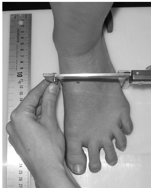
Figure 3 Use of modified digital caliper to measure midfoot width in weight bearing.
